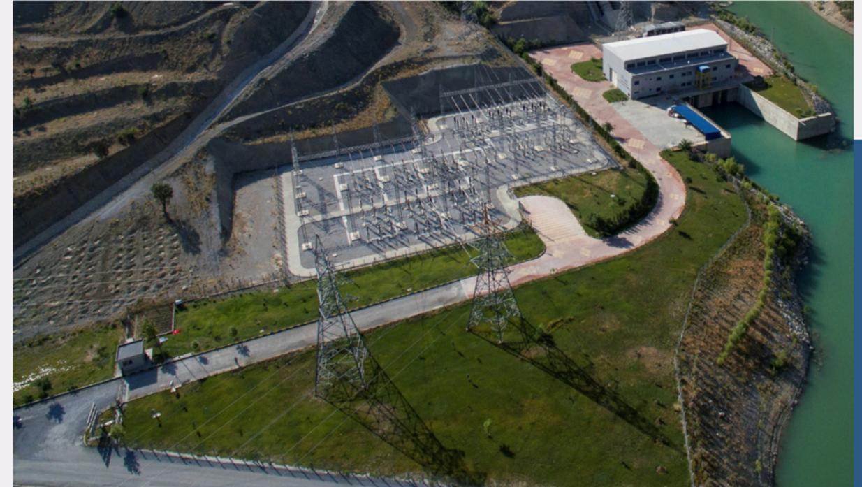
Starting operation in 2011, Hacınınoğlu HEPP is located in Kahramanmaraş, in the Ceyhan Basin. The plant is connected to TEİAŞ' Kılavuzlu and Narlı switchyard of 154 kV, and has an installed capacity of 142 MW.
